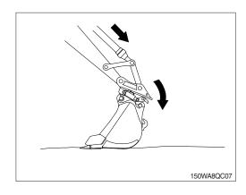
(10) To engage the quick coupler, release the quick coupler button on the right RCV lever.
